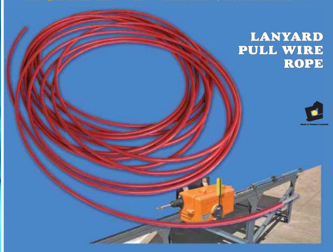
SAFE-T-LANYARD Stainless Steel Pull Wire Rope is a UV Stable Red Polyurethane coated 304 Stainless Steel 3mm ID x 5mm OD 6 x 19 construction wire rope, designed and manufactured for the purpose of a lanyard emergency stop pull wire system.
