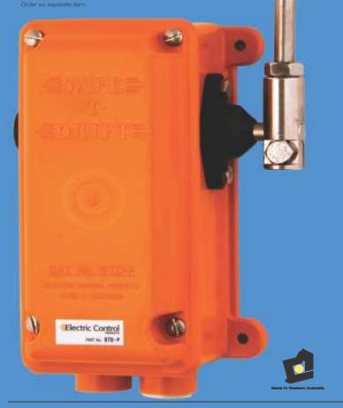
The **SAFE-T-DRIFT** Heavy Duty Belt Misalignment Switch, is made for applications requiring a unit which caters for high speed belt applications, having a pre-warn trip contact and a final trip contact, both individually adjustable.
